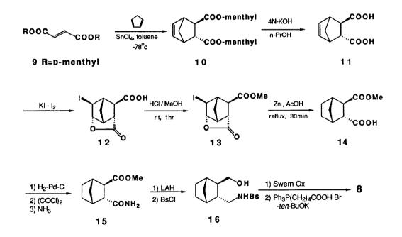
gaseous ammonia. Simultaneous reduction of both amide and ester moieties in 15 with lithium aluminum hydride in THF at reflux for 3 h, followed by selective sulfonylation of amino function with p-bromobenzenesulfonyl chloride gave 16 (60% from 15). The  $\alpha$ -side chain was introduced by the following sequence. After Swern
